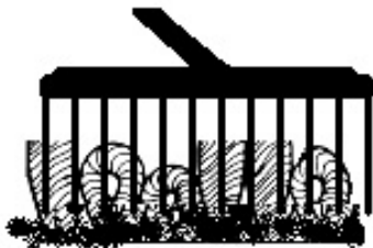
Figure 3 Grooming - Soils now in Solution "Appears" Clean
