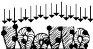
Figure 2 Soiled Fabric Being Pre-conditioned with High Pressure, Hot Water & Fitting Detergent
